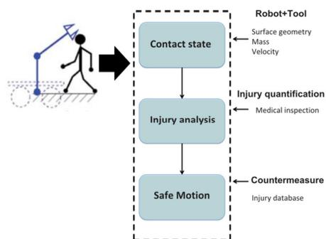
Figure 1 – Medical evaluation based on mass, velocity, and surface geometry to ensure safe motion behavior
